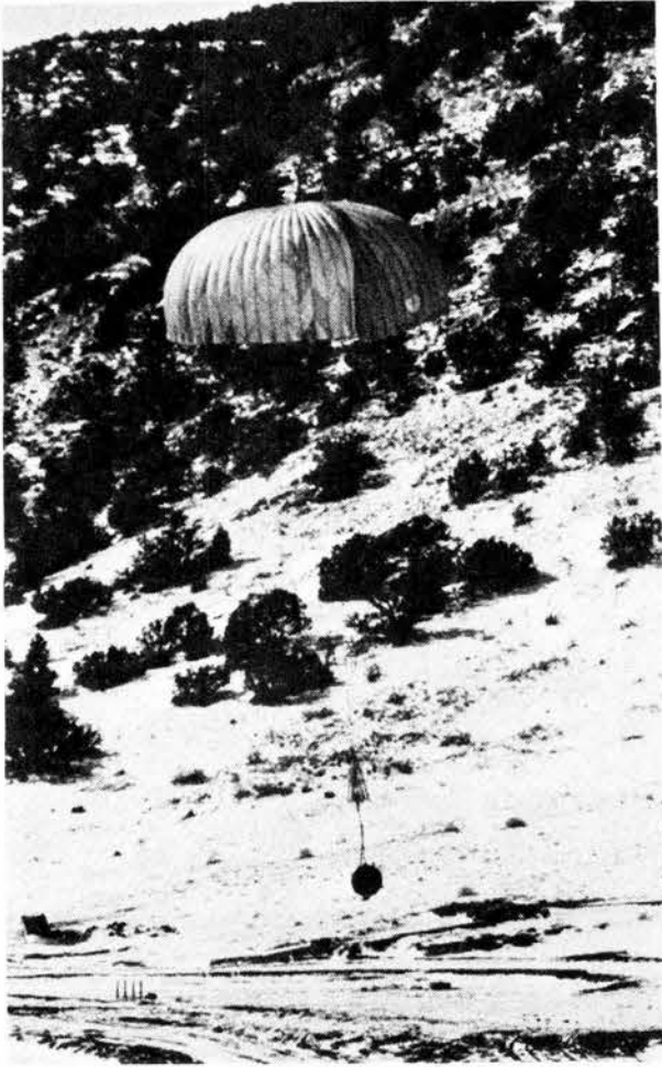
RETROROCKETS OF THE RAPID system stopped a 5000-pound sphere in mid-air and gently lowered it to impact during a drop test recently from the Sol Se Mete aerial cable facility in Coyote Test Field.
